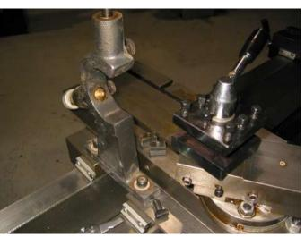
5. Installed follow rest shown from the tailstock.
