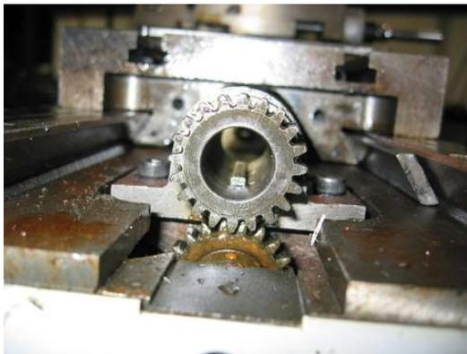
4. Remove the key (#22). Rotate the gear (#23) to
