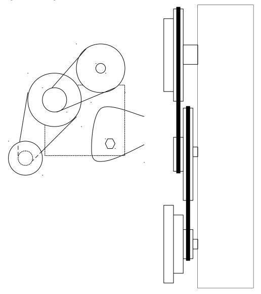
4.To go back to the faster speeds, remove the two belts and reinstall the single belt. The single belt may ride on one side of the speed reducer pulley and make it turn also. This is normal and will not cause any problems.
