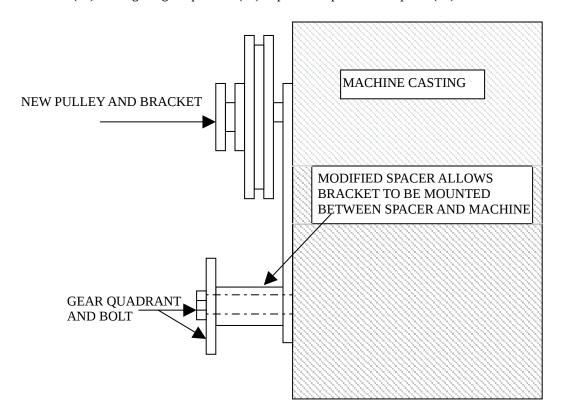
2.Reassemble the quadrant with the modified spacer and the new bracket mounted against the machine as shown above.
