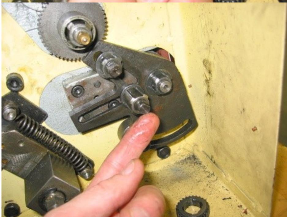
Fig 6 – B/C gears mounting shaft has a t-slot back. When the shaft is loosened, it will slide left and right and allow the B/C gear to mesh with the D gear.
