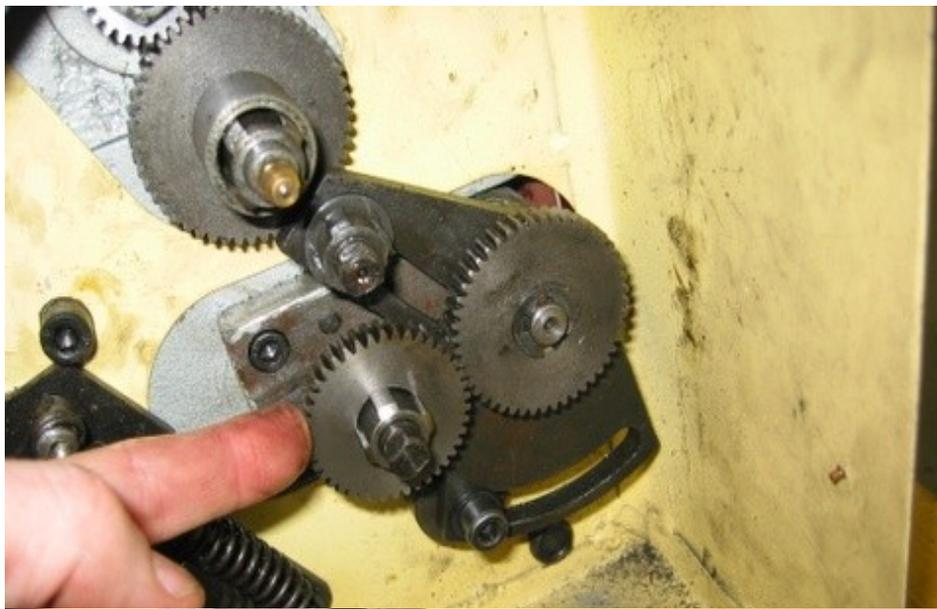
Fig 13 – Slide the C gear so it meshes with the D gear.
