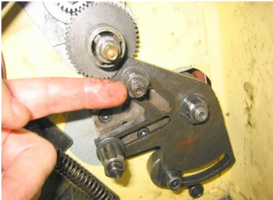
Fig 10 – E gear shaft run all the way up and locked in place. Splined hub, C30081S is installed.
