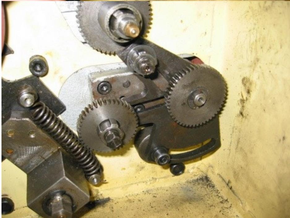
Fig 12 – Install the C gear on the B/C gear shaft.
