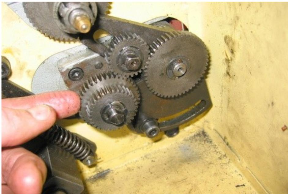
Fig 22 – Since the E gear is simply acting as a bridge, the number of teeth is not critical. Use a gear that fits well in the space.
