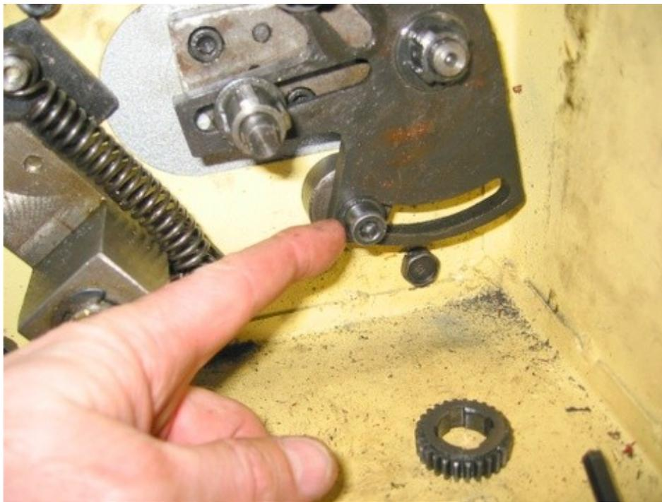
Fig 4 – Remove all the gears. Loosen the socket head cap screw and allow the mounting plate to move.
