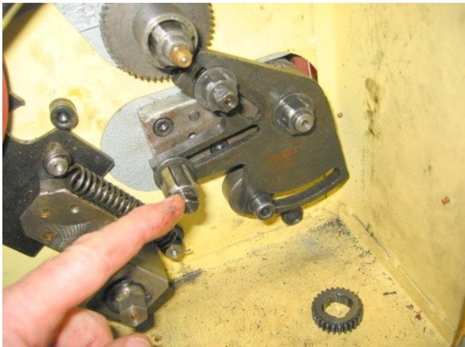
Fig 7 – The spline hub, C30081, goes on the shaft. Finger is pointing to the B/C shaft
