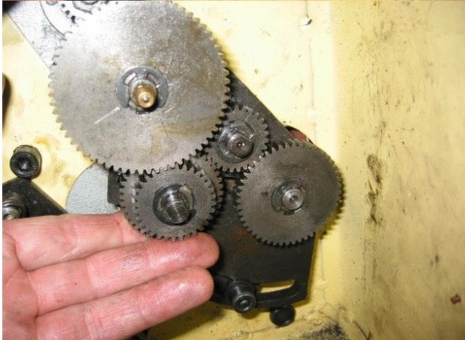
Fig 23 – Once the E gear is locked in place, lock the B/C gear shaft and rotate the mounting plate to mesh A and B. Tighten the socket head cap screw.
