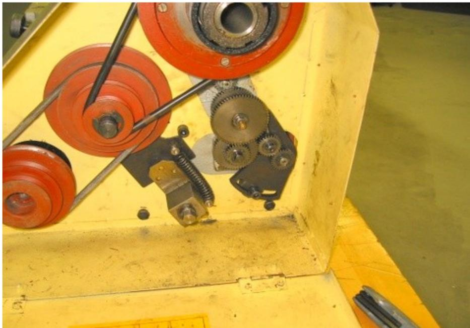
Fig 1 – Standard 5-gear setup
