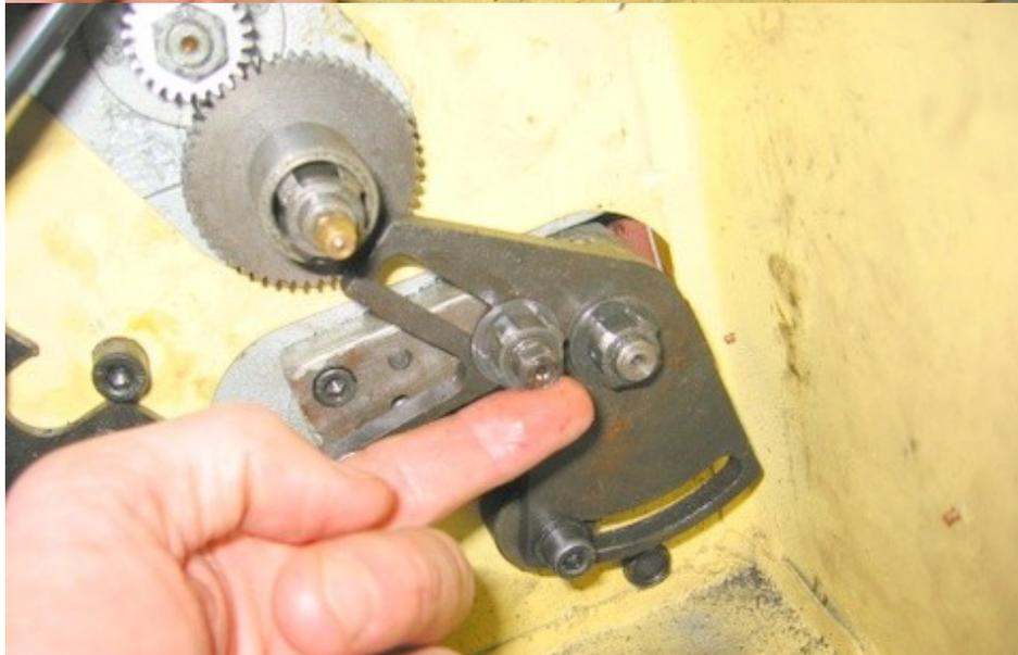
Fig 8 – The E gear shaft is above the B/C gear shaft. It allows LH threading and bridges some gear combinations.
