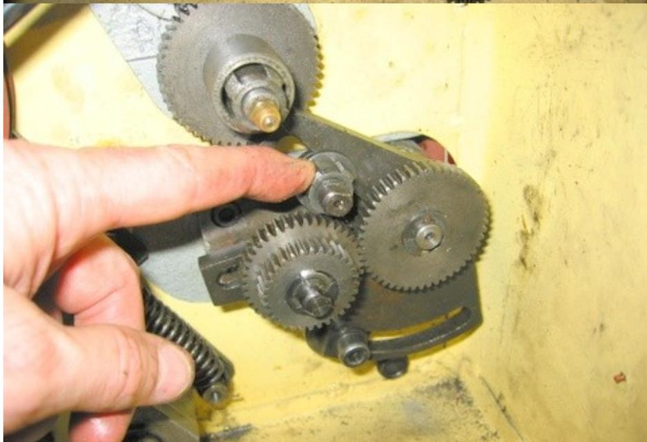
Fig 17 – If the E gear shaft interferes with the gears, slide it to the end of its travel and lock in place.
