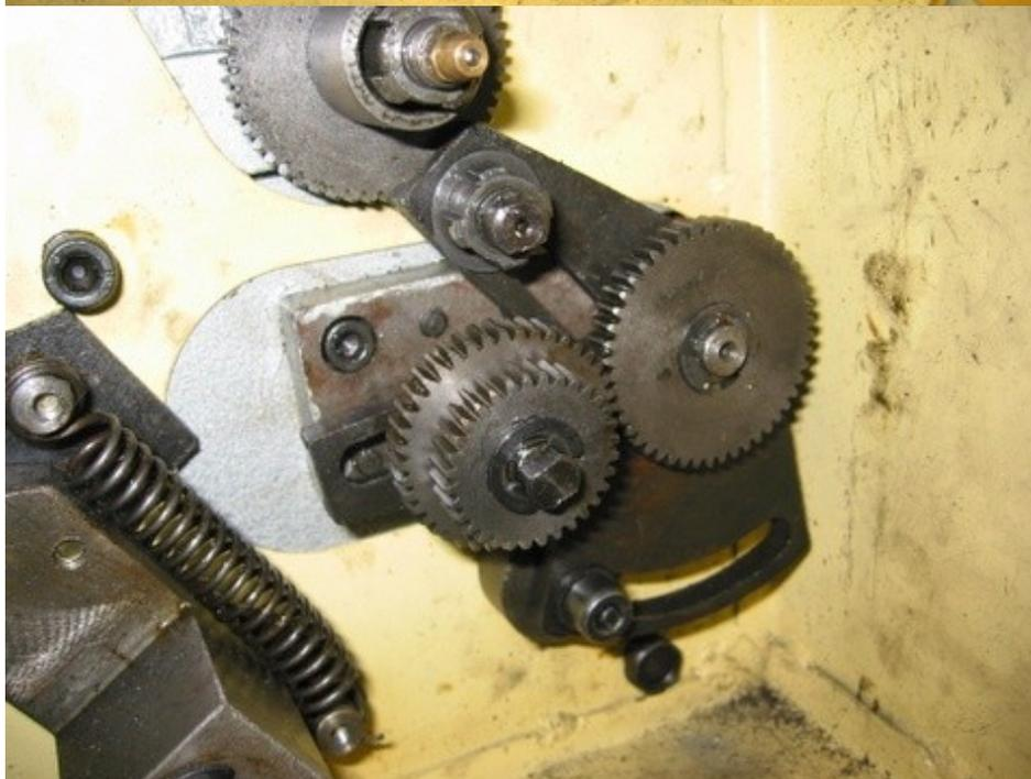
Fig 15 – B and C gears are installed, shaft locked in place and C-clip installed. It is often easier to install the C-clip, then mesh the gears, then lock the shaft in place.
