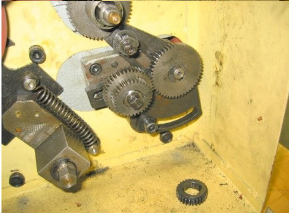
Fig 14 – Install the B gear on top of the C gear. The B gear can be larger than the C gear and can hide it when installed.
