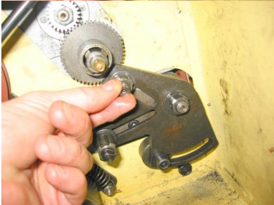
Fig 9 – The E gear shaft moves like the B/C gear shaft. The upper corner of the mounting plate may require some grinding to fit past the A gear shaft.
