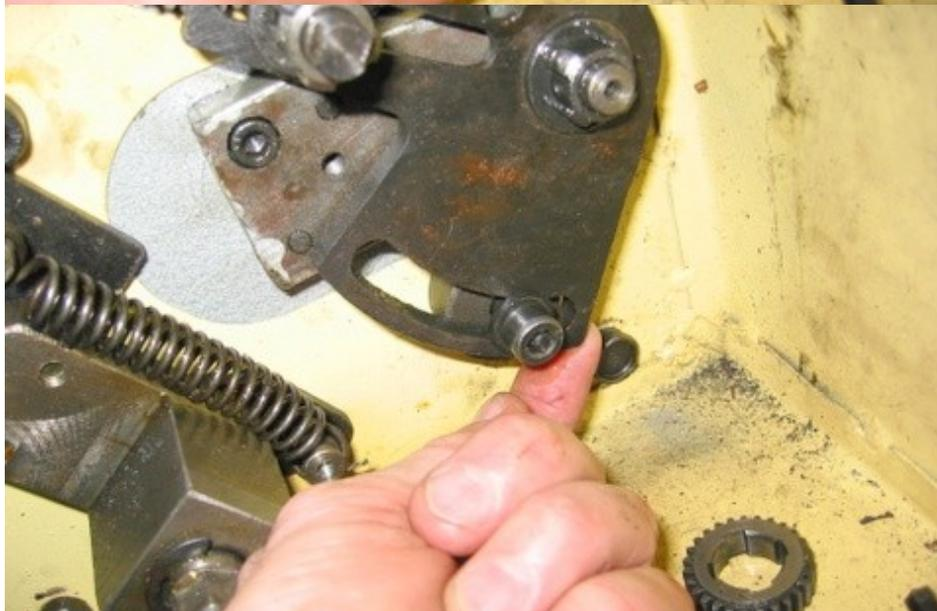
Fig 5 – The plate will move in the radius slot and will bring the A and B gears together when they are installed.
