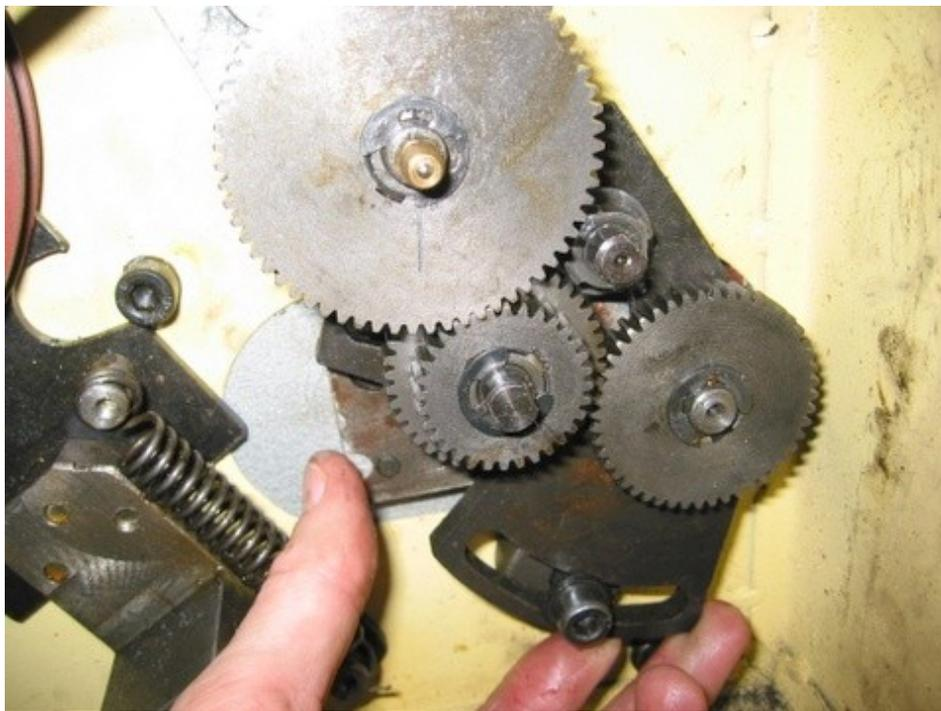
Fig 19 – Install the A gear and then the C-clip. Rotate the mounting plate until the A and B gears mesh.
