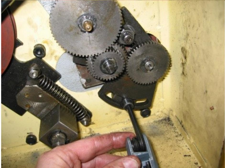
Fig 20 – Tighten the socket head cap screw to lock the gears in place
