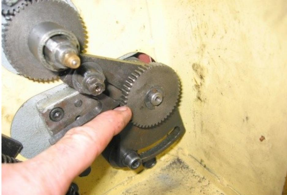
Fig 11 – Install the D gear first and put the C-clip in place. The D gear requires a splined hub to mount on the shaft. Use C30081S or C30081S-1.
