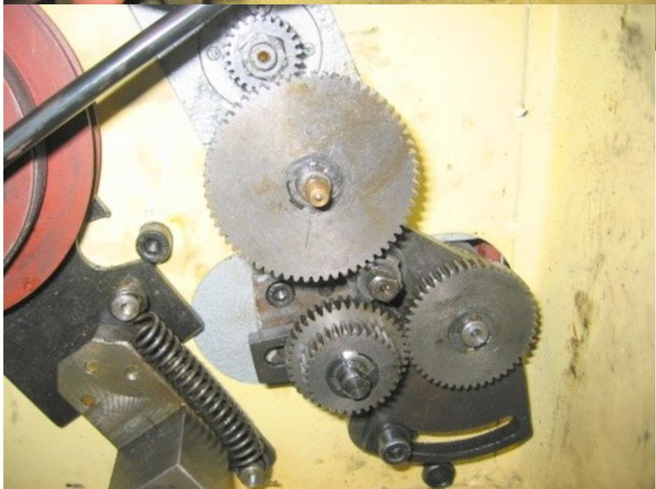
Fig 18 – Install the A gear and install the C-clip to keep it in place.
