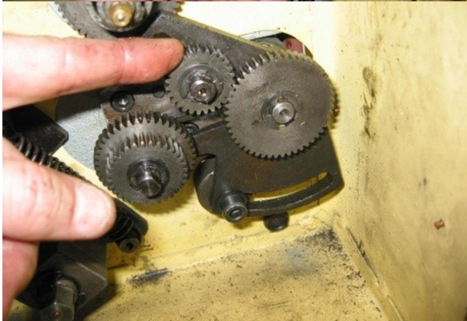
Fig 21 – **E-gear install.** At times you may need to install the E-gear to bridge between the D gear and the C gear.
