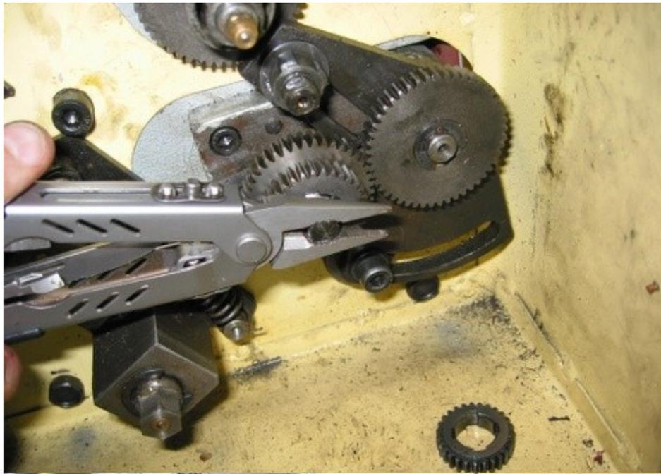
Fig 16 – Tighten the B/C shaft to lock the gears in place.
