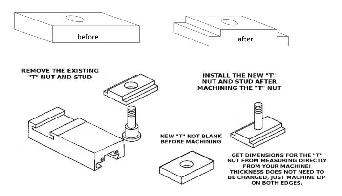
Slide the machined "T" nut and stud assembly into the top of the slide of the tool post.
