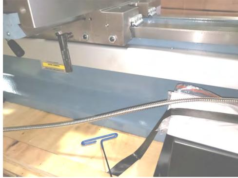
**Step 5:** Install the rectangular bracket on the underside of the carriage table just above the X-Axis Encoder Bracket using the M5 x 20mm screws.
