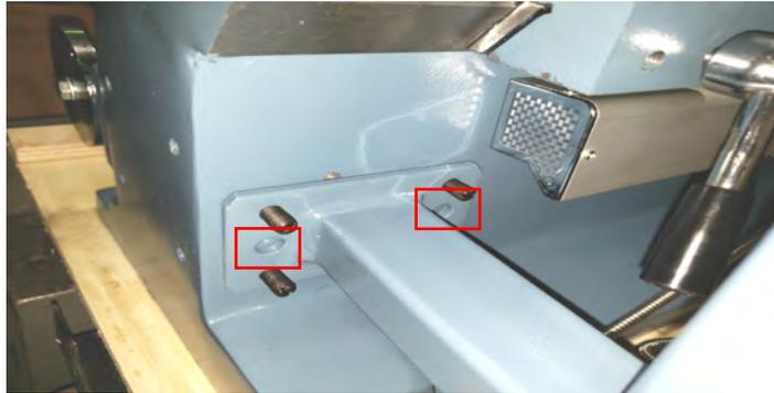
**Step 2:** Once the holes are marked, punch to center punch the holes. Drill and tap the holes to 8mm. Assemble the display arm.
