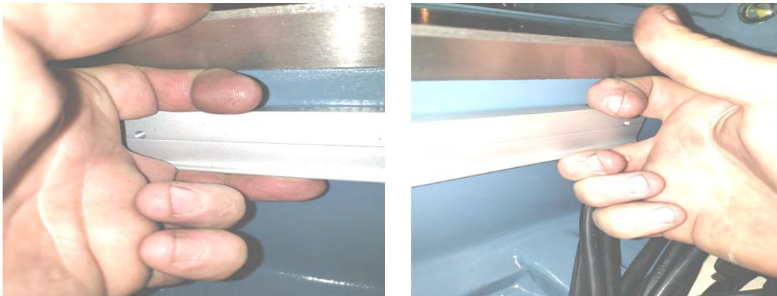
**Step 2:** Remove the red shipping braces from the X-Axis Encoder by unscrewing the screws that are holding them in place.
