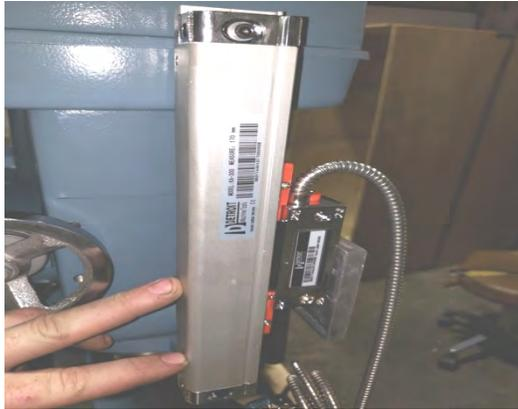
**Step 6:** Line the reader up with the square bracket by lightly tapping on the square bracket with a hammer, as pictured, to move the mounting bracket closer to the reader on the encoder.
