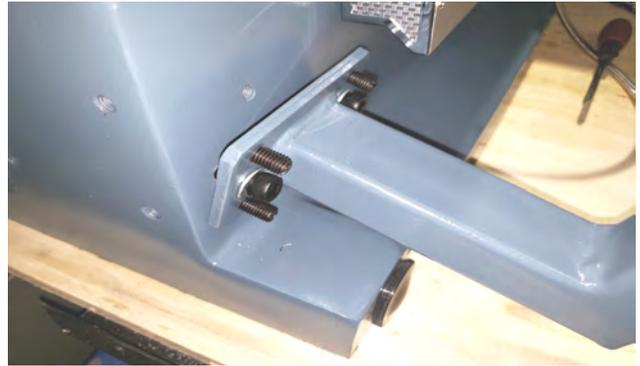
**Step 3:** Assemble the display brackets and pins, as pictured below.
