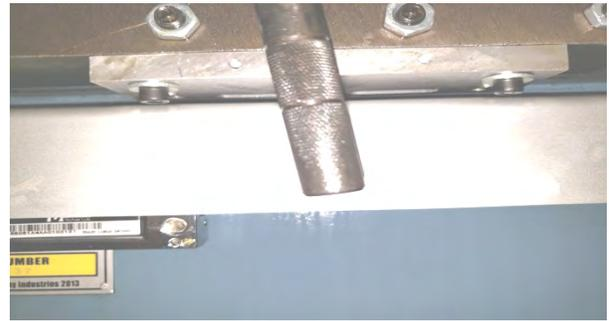
**Step 6:** Install the slotted square bracket onto the rectangular bracket as shown below. Use the M4 screws.
