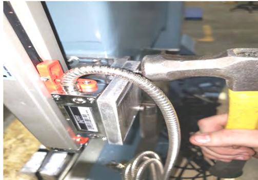
**Step 7:** Mount the reader to the square bracket and remove the red shipping blocks.
