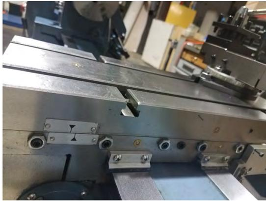
**Step 2:** Install the Y-Axis Encoder Bracket to the table using the two shortest 5mm allen head screws. Make sure the bracket is up as high as it can go while also aligned with the top of the table.
