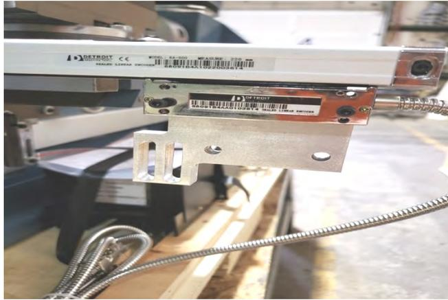
**Step 5:** Slide the Encoder over and start the screws to mount the bracket to the outside holes in the side of the saddle/carriage using the M6 x 16mm screws.
