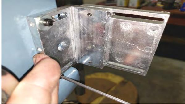
**Step 4:** Install the Z-Axis Encoder Bracket using two more 4mm screws that are 10mm long (they are shorter than the others). Screw them into the end of the already-installed Quill Bracket.
