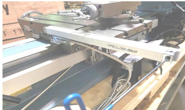
**Step 4:** Install the L-Shaped Bracket onto the Y-Axis Encoder using the M3 screws.
