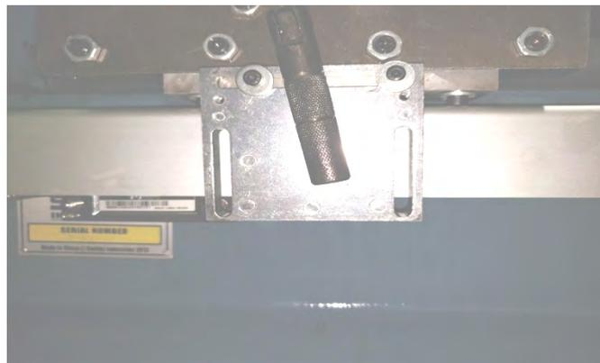
**Step 7:** Install the angle bracket onto the slotted square bracket and connect it to the reader part of the encoder using the M4 x 16mm screws.
