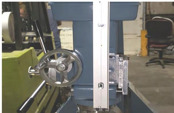
**Step 5:** Mount the Z-Axis Encoder onto the Z-Axis Encoder Bracket using the extra-long 4mm capscrews on either end of the encoder. These capscrews are included with the encoder.
