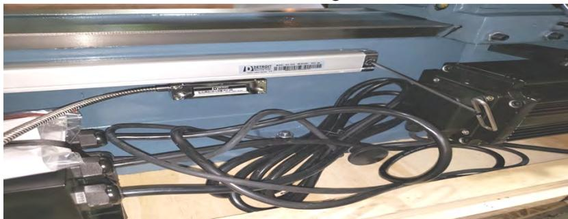
**Step 4:** Install the X-Axis Encoder Cover using the flathead 3mm screws. It must be installed at this point – it will not fit after the next steps are completed.
