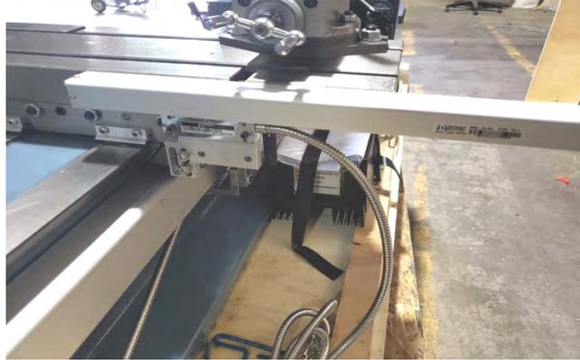
**Step 1:** Clean the table so that it is free of any debris. Make sure the oil buttons on the table are flush on the two sides and the top. If they aren't, use a very flat punch and hold it flat. Using a round surface such as a hammer will ruin the oil button.
