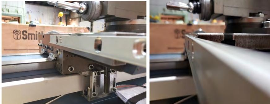
**Step 3:** Install the Y-Axis Encoder onto the Y-Axis Encoder Bracket using the M3 screws that came in the bag with the encoder.
